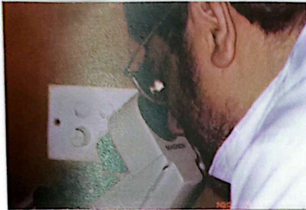
Fig. 6.10 Dioptric power and axis of the cylinder of spectacle lenses is being verified with a lensometer
